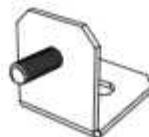
Side Panel to Frame Bracket 064.1022 x4
